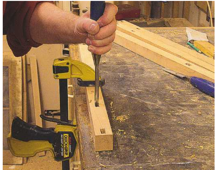
▲ Pic.7 Cut the mortises to finished sizes using chisels. The mortises will break into each other as they are cut into adjacent faces on the legs
